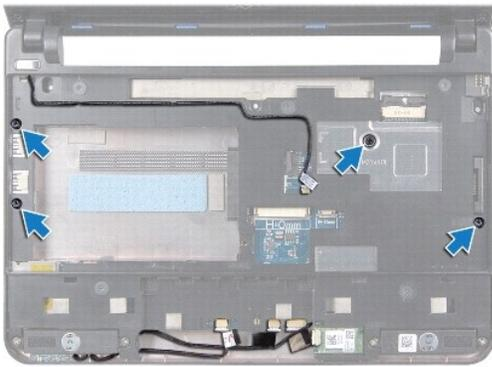
9. Disconnect the power button cable, Bluetooth card cable, power/battery status light cable, and speaker cable from their respective system board connectors.
